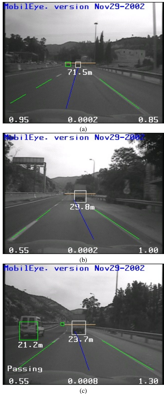
Figure 3: A typical sequence where the host vehicle decelerates so as to keep a safe headway distance from the detected vehicle. The detected target vehicle (the truck) is marked by a white rectangle. As the distance to the target vehicle decreases the size of the target vehicle in the image increases.
