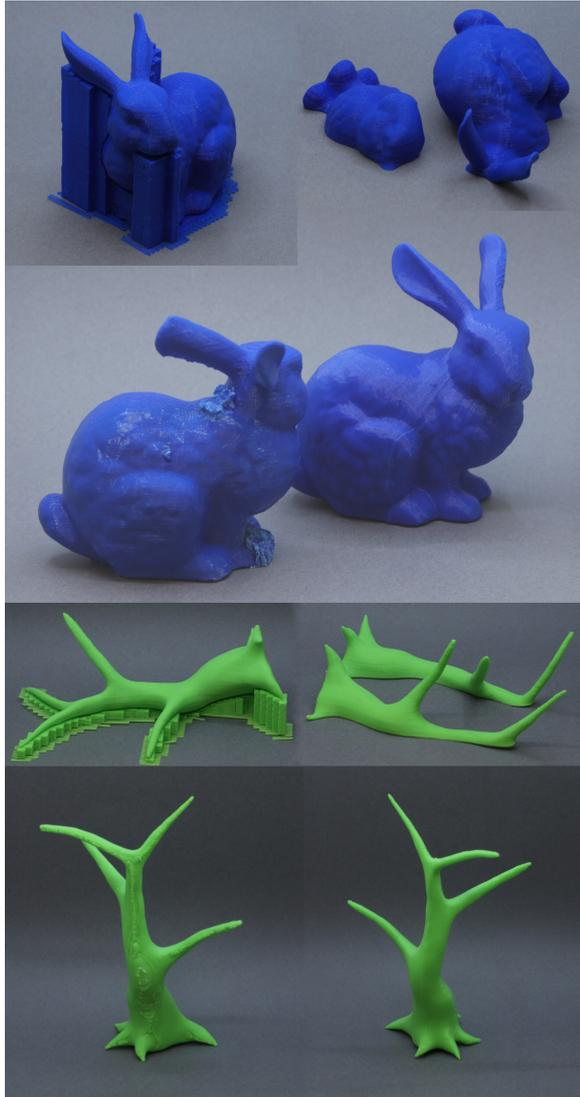
**Figure 12:** A visual comparison showing the region where the support structures were removed, next to the glued seam appearing in our result.
