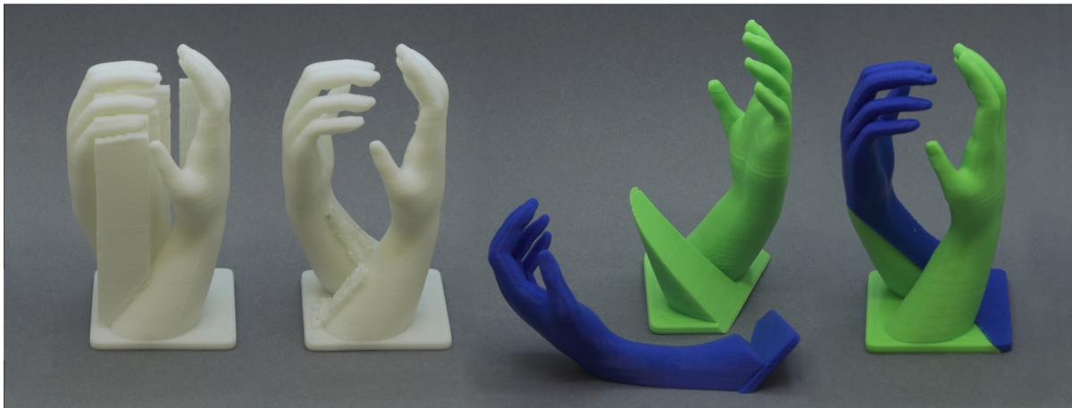
**Figure 1:** An object requiring support when printed by an FDM printer. Two left images show the object with support structures and after their removal by a craft knife. Removal marks are clearly seen despite the elaborate effort put. Partitioning the object by a single plane of a precise location and angle results in two printable subparts. Gluing the two results in a cleaner surface, 20 minutes shorter printing-time, and saves 70cm of filament.
