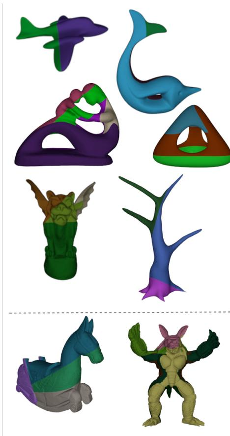
**Figure 11:** Rendered images of partitions produced by our method. Objects on the top were partitioned with  $\theta_{crit} = 135^\circ$  and the bottom ones with  $\theta_{crit} = 150$ . The different subparts are encoded with distinct colors.
