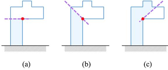
**Figure 4:** Base Extraction steps. The first iteration (a) encounters a non-printable edge (with red). The second step (b) corrects the angle and increase the printable volume. The third step (c) increases the printable subpart up to the point where the cutting-plane reaches  $\theta_{crit}$  and will produce non-printable faces if rotated any further.
