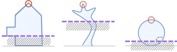
**Figure 5:** Three examples showing the printable subpart found by the tip extraction procedure. Assuming  $\theta_{crit} < 135^\circ$ , each of these solutions are optimal, or appear in the optimal solution.
