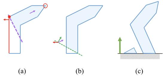
**Figure 6:** Tip Extraction steps. The first iteration (a) encounters a non-printable face (marked in red). The second step (b) brings the cutting-plane's normal closer (as shown by green arrow) to that of the limiting face (red), and thereby increases the printable volume. The resulting parts are printable as shown in (c). For this example to be realistic assume  $\theta_{crit} = 135^\circ$ .
