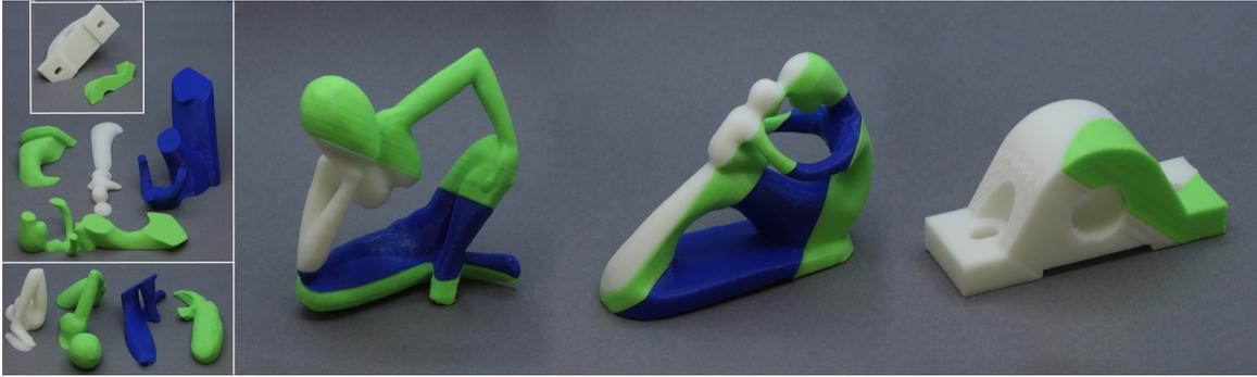
**Figure 10:** 3D printed objects. Different PLA colors are used for revealing the different subparts, which are shown before gluing on the right. A critical angle of  $\theta_{crit} = 150^\circ$  was used in these examples.
