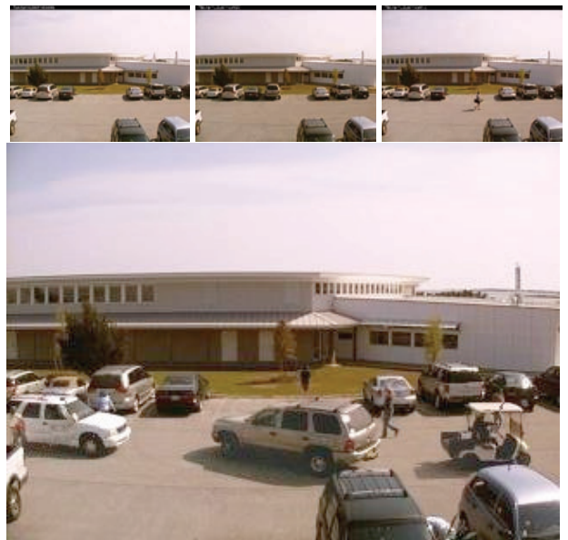
Figure 8. Top: Three images taken over several hours from a webcam watching a very quiet street Bottom: A frame from a 1 minute synopsis of this period. In this synopsis we have given a high score to phase transitions (e.g. moving objects that stop and become background), so the video synopsis includes mostly cars being parked or pulling out of parking.
