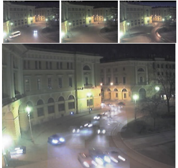
Figure 7. Top: Three images taken overnight from a webcam in St. Petersburg Bottom: A frame from a 1 minute synopsis of this period. While this street is very busy during the day, it is practically deserted during the night. The video synopsis brings together many cars that passed this street during different times.
