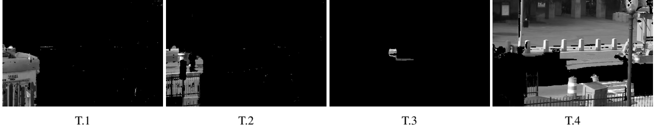
Figure 9: The tram example from the ChangeDetection.net dataset. A tram is initially at rest at the station and later moves off. A package is left on the sidewalk about 40% into the sequence. T.1 shows the parked tram ( \tau = 33\% ). T.2 shows the area behind the parked tram ( \tau = 56\% ). T.3 shows the left package ( \tau = 58\% ). T.4 shows the scene background ( \tau = 93\% )
