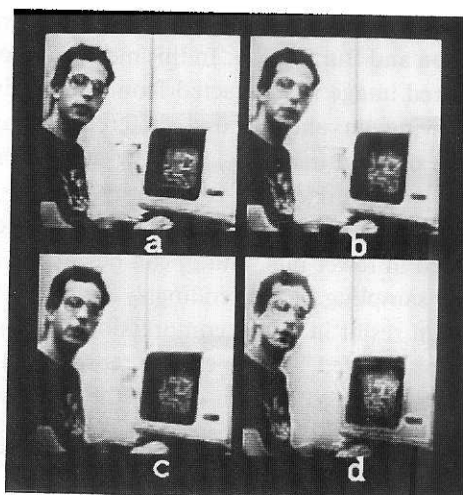
Fig. 2. Compression using the Laplacian pyramid. (a) Four quantization steps at all levels (2.66 bits/pixel), (b) Two steps at the lowest level, four steps at all other levels (1.66 bits/pixel), (c) Two steps at the lowest level, eight at all other levels (2 bits/pixel), (d) Two steps at all levels (1.33 bits/pixel).
