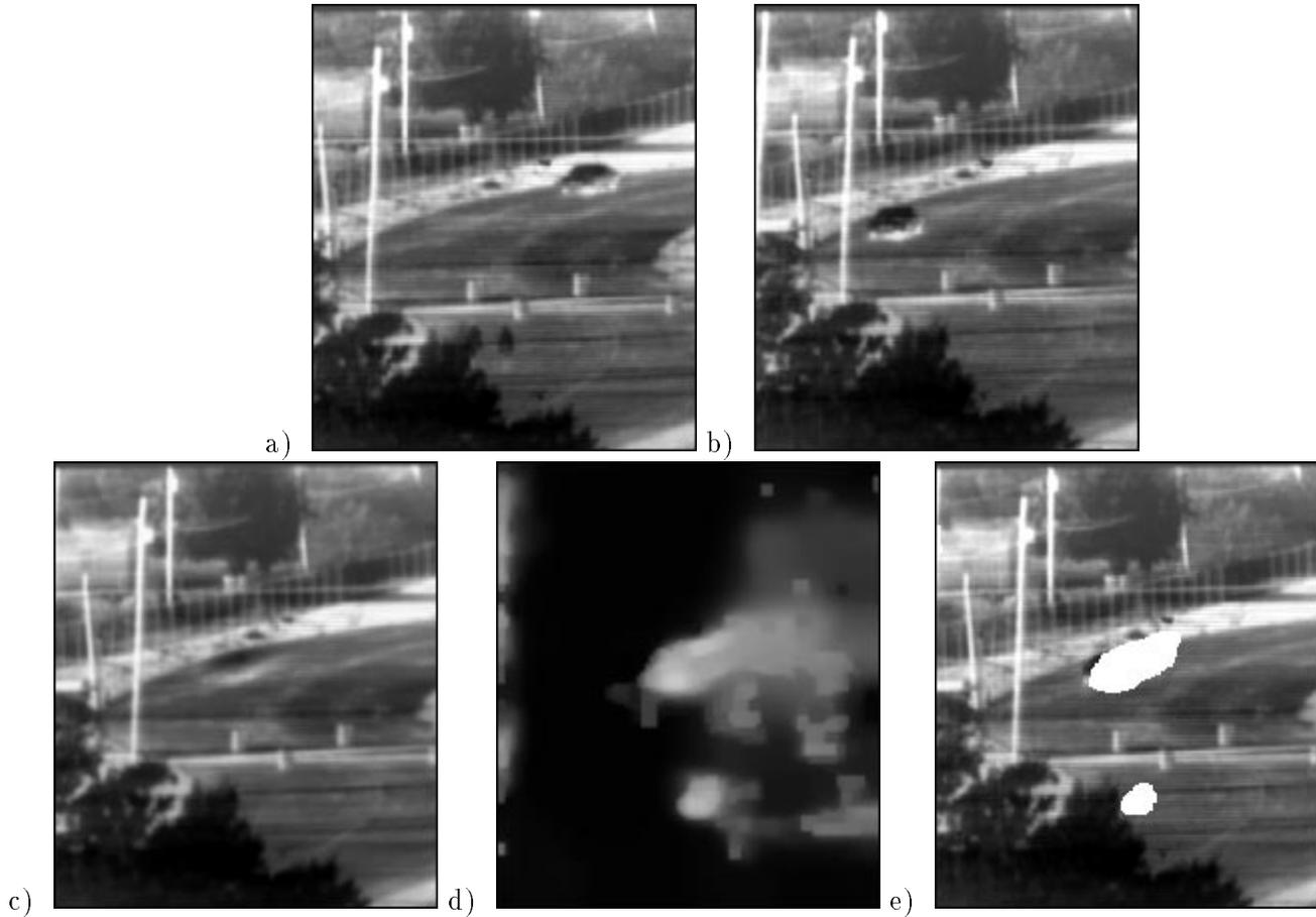
Figure 3: Detecting and tracking the dominant object in an infrared image sequence using temporal integration.
