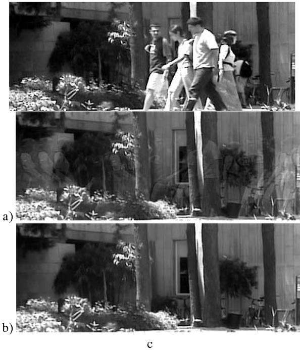
**Figure 4.** The results on the “University” sequence. a) A patch from one of the input images. b) The IBP algorithm. c) The proposed median IBP algorithm.
