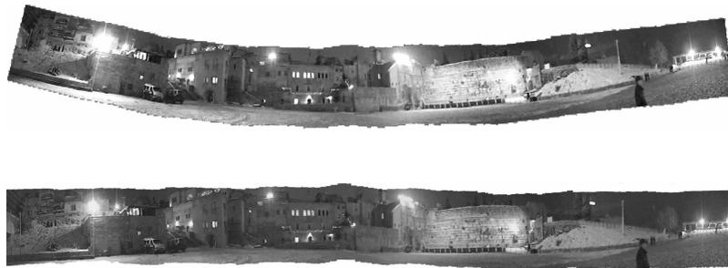
FIGURE 14. Mosaicing from a panning camera which is slightly tilted upward. Regular mosaicing results in a curled image, while rectified mosaicing results in a straight mosaic.
