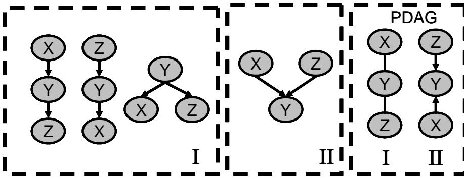
Figure 2.3: The skeleton  $X - Y - Z$  is partitioned into two equivalence classes: I representing  $((X \perp Y | Z), \neg(X \perp Z | \emptyset))$  and II the v-structure representing  $\{\neg(X \perp Y | Z), (X \perp Z | \emptyset)\}$ . The right pane illustrates the corresponding PDAGs.
