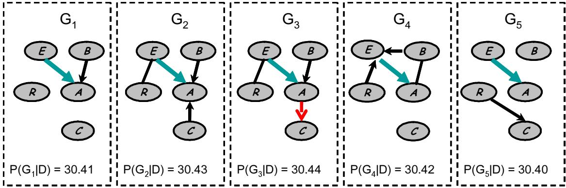
Figure 3.2: An ensemble of high scoring networks: Presented are five different Bayesian networks. The score of the network with respect to the dataset  $D$  is listed below each network. While  $\mathcal{G}_3$  is the highest scoring network, the other networks are almost as likely. The edge  $A \rightarrow C$  exists in  $\mathcal{G}_3$ , but it is absent from all other high scoring networks. On the other hand, all five networks agree on the edge  $E \rightarrow A$ .
