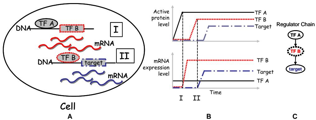
Figure 7.1: Regulator chain  $A \leftrightarrow B \leftrightarrow C$  (A) Cartoon of the cell at two time points. At time I, transcription factor (TF) A activates transcription factor B, raising the levels of mRNA and protein for transcription factor B. In time II, transcription factor B activates its target. (B) Time series plotting the protein and mRNA levels. (C) Network motif. The gene with the dotted border is predicted as regulator.
