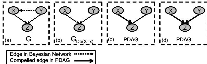
Figure 4.6: v-structures in  $\mathcal{G}_{do(m)}$  are compelled: (a)  $\mathcal{G}$  does not have a v-structure. (b)  $Y \rightarrow X$  is removed in  $\mathcal{G}_{do(X=x)}$  creating a v-structure. (c) The edge  $X \rightarrow Z$  is adjacent to a mutated variable and thus compelled by Theorem 4.2.4. (d) The edge  $Y \rightarrow Z$  is compelled by the second propagation rule in Figure 2.4
