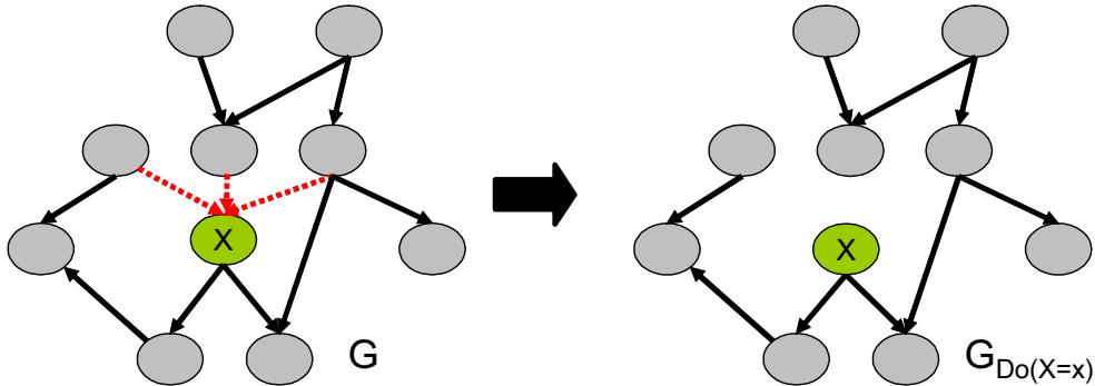
Figure 4.5: Example of ideal intervention: Assume the variable  $X$  is mutated in  $\mathcal{G}$ . We construct the corresponding  $\mathcal{G}_{do(X=x)}$  by removing all edges incoming from  $\text{Pa}_X$  (red edges)
