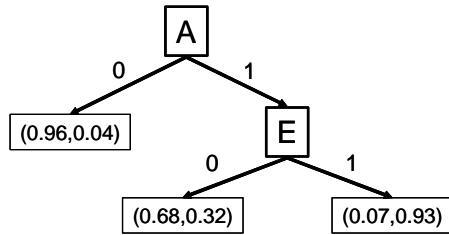
Figure 2.2: An example of a tree-CPD. Each square represents a query on a variable ( $A$  and  $E$ ). Each edge is annotated with the value of its associated query node. The leaves contain probability distributions. Notice that when  $A$  is off, the value of  $E$  does not matter
