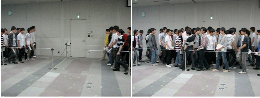
Fig. 3. Experiments on facing groups: several experiments were conducted on real pedestrian dynamics, some of which also considered the presence of groups of pedestrians, that were instructed on the fact that they had to behave as friends or relatives while moving during the experiment.
