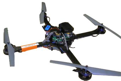
Figure 1: Ascending Technologies Hummingbird UAV
