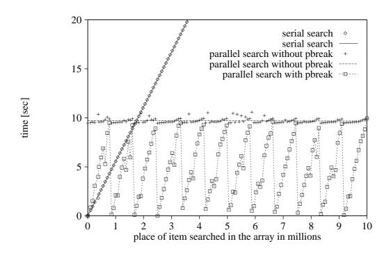
Figure 7: Results of searching for an element in a large array.
