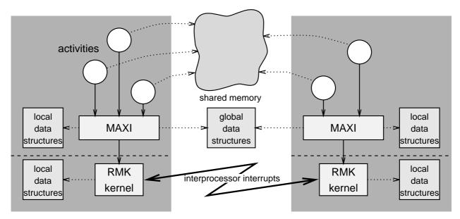
Figure 2: Interactions among components of the application and MAXI. Solid vertical arrows denote system calls, and dotted arrows denote access to data structures.
