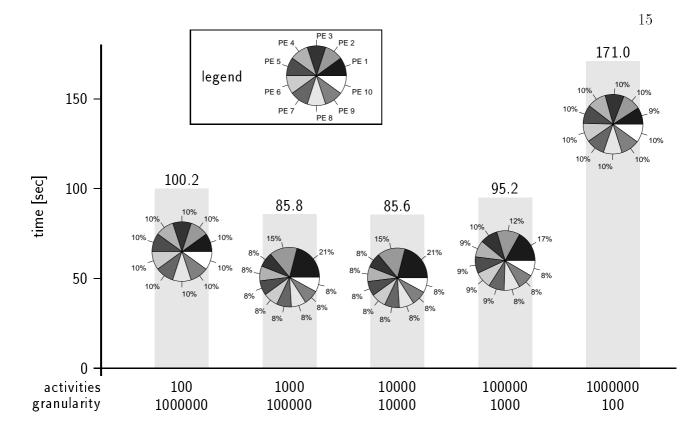
Figure 4: Results of load balancing experiment. The time is the parallel completion time. Percents do not always add up to 100 because of rounding error. It is therefore best to divide 100,000,000 operations into several thousand activities when 10 processors are used.
