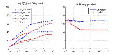
Fig. 4. The delay and throughput behavior achieved by a two-burst MBT protocol with  ${\bf v}=[2,4],$  with and without coding. Channel is i.i.d. with  $\rho=0.5$  and  $d_c=10.$
