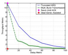
Fig. 3. The delay-throughput tradeoff for optimized MBT and truncated ARQ, compared to the genie-assisted bound and to the SUA scheme. ARQ performance is not shown, since it yields  ${\rm DM}=\infty$ . Channel is i.i.d. with  $\rho=0.5$  and  $d_c=10$ .
