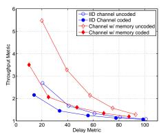
Fig. 5. The delay-throughput tradeoff for channels with and without memory, using MBT protocols with and without coding,  $d_c=10$  and  $\rho=0.5$ .
