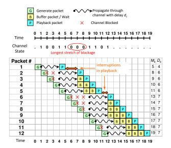
Fig. 2. Example of genie-assisted system operation with  $d_c = 3$ .
