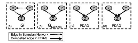
Figure 4.6: v-structures in  $\mathcal{G}_{do(m)}$  are compelled: (a)  $\mathcal{G}$  does not have a v-structure. (b)  $Y \to X$  is removed in  $\mathcal{G}_{do(X=x)}$  creating a v-structure. (c) The edge  $X \to Z$  is adjacent to a mutated variable and thus compelled by Theorem 4.2.4. (d) The edge  $Y \to Z$  is compelled by the second propagation rule in Figure 2.4
