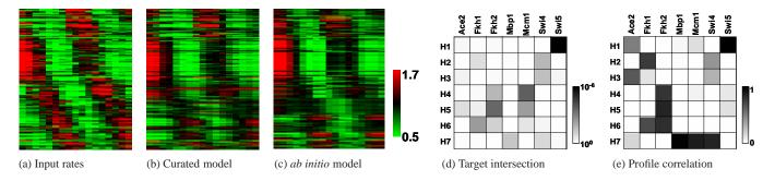
**Fig. 5.** Comparison of *ab initio* structure learning vs. parameter learning for the curated cell cycle regulatory diagram. (a) Measured transcription rates for 141 genes. (b) Predicted rates in the curated model after learning parameters. (c) Predicted rates after *ab initio* structure learning. (d) log *p*-value of target intersection groups between known and *ab initio* regulators. (e) Positive correlations between learned activity profiles of known and *ab initio* regulators.
