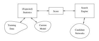
Figure 2: Architecture of the implementation of the MS-EM algorithm.
