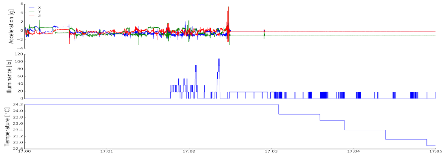
Fig. 1. Raw data as recorded by the smart-watches, including tri-axial accelerometer (top panel), light sensor (middle), and temperature (bottom). This plot shows data from a single patient, recorded on 28 Jan, 2017 at 5:00-5:05pm. Only accelerometer data was used for further analysis.
