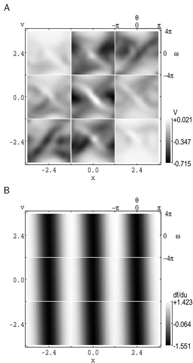
Figure 9: (A) The landscape of the value function for the cart-pole swing-up task. (B) The learned gain model  $\frac{\partial \dot{\omega}}{\partial u}$ .
