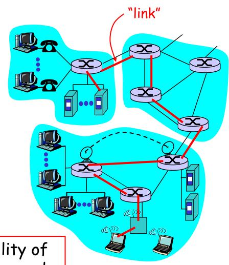
data-link layer has responsibility of transferring datagram from one node to adjacent node over a single link
