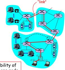
data-link layer has responsibility of transferring datagram from one node to adjacent node over a single link
