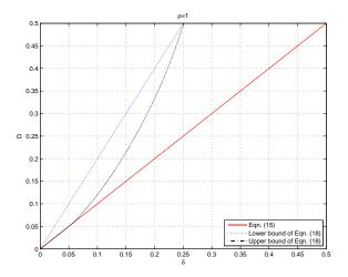
Fig. 1. Trade-off between  $\delta$  and D in a BSSC( $\delta$ ) for  $\rho=1$ . An identity map (single-letter scheme) is everywhere optimal.
