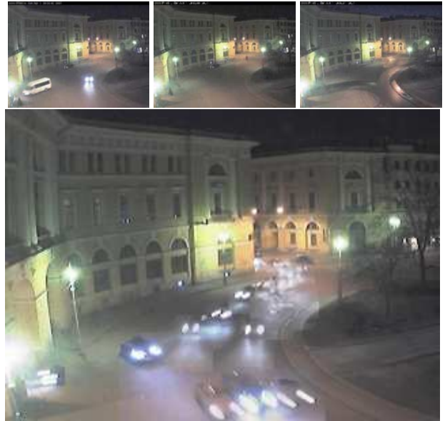
Figure 8. Top: Three images taken overnight from a webcam in St. Petersburg www.opentopia.com/showcam.php?camid=4567 . Bottom: A frame from a 1 minute synopsis of this period. While this street is very busy during the day, it is practically deserted during the night. The video synopsis brings together many cars that passed this street during different times.
