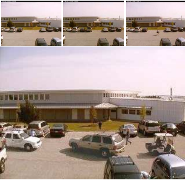
Figure 9. Top: Three images taken over several hours from a webcam watching a very quiet street www.opentopia.com/showcam.php?camid=3931 . Bottom: A frame from a 1 minute synopsis of this period. In this synopsis we have given a high score to phase transitions (e.g. moving objects that stop and become background), so the video synopsis includes mostly cars being parked or pulling out of parking.
