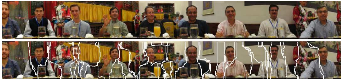
Fig. 18. When the camera is translating, the dynamics in the scene consists of both moving objects and the parallax. Both are treated in the same manner using the 4D min-cut. Gradient domain composition [1] handled variations in illumination. (top) A frame from panoramic movie (the entire video clip is available at www.vision.huji.ac.il/dynmos ) (bottom) The min-cut avoids stitching inside moving objects or inside foreground objects (which have high disparity due to parallax).
