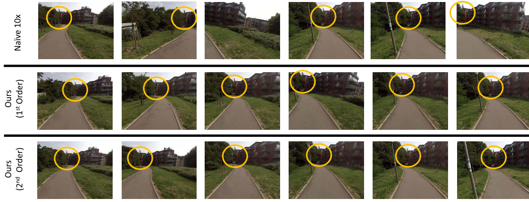
Fig. 5. Comparative results for fast-forward from naïve uniform sampling (first row), EgoSampling using first-order formulation (second row) and using second-order formulation (third row). Note the stability in the sampled frames as seen from the tower visible far away (yellow circle). The first-order formulation leads to a more stable fast-forward output compared to naïve uniform sampling. The second-order formulation produces even better results in terms of visual stability.
