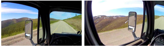
Fig. 12. Failure case for the proposed method showing two sample frames from an input sequence. The frame-to-frame optical flow is mostly low because of distant view and (relatively) static vehicle interior. However, since the driver shakes his head every few seconds, the average optical flow magnitude is high. The velocity term causes us to skip many frames until the desired K_{\text{flow}} is met. Restricting the maximum frame skip by setting \tau to a small value leads to arbitrary frames being chosen looking sideways, causing shake in the output video.
