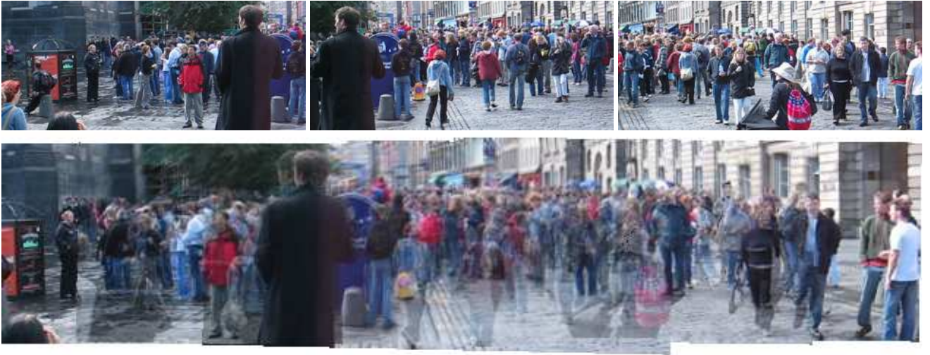
Figure 5. While the dynamic crowd in this festival makes alignment a real nightmare, predictive alignment had no problems. Three original frames are shown at the top. The panorama is stitched from the video after alignment by frame averaging. The scene dynamics is visible by ghosting, and the static background is clearly well registered.
