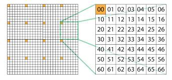
Figure 2: An example matrix layout for CAPS. Each of the 16 submatrices as shown on the left has exactly the same layout. The colored blocks are the ones owned by processor 00. On the right is a zoomed-in view of one submatrix, showing which processor, numbered base 7, owns each block. This is block-cyclic layout with some blocksize b, and matches our layout requirements with parameters  $(n=4\cdot 49\cdot b, P=49, s=2)$ .
