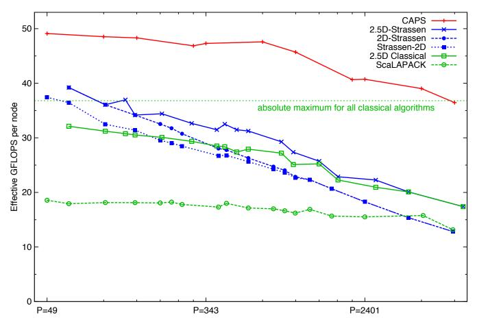
Figure 3: Strong scaling performance of various matrix multiplication algorithms on Cray XT4 for fixed problem size n=94080. The top line is CAPS as described in Section 3, and substantially outperforms all the other classical and Strassen-based algorithms. The horizontal axis is the number of nodes in log-scale. The vertical axis is effective GFLOPS, which are a performance measure rather than a flop rate, as discussed in Section 5.2. See Section 5.4 for a description of each implementation.
