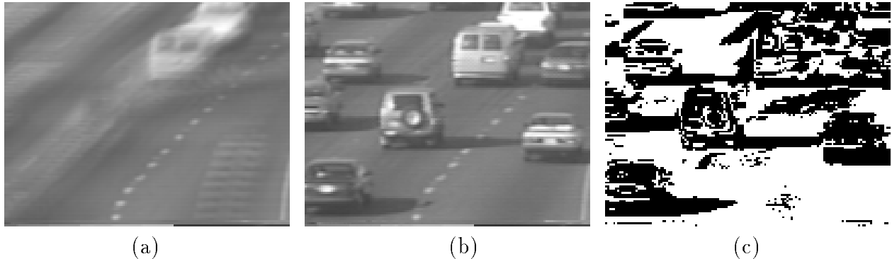
Figure 2: (a) Background image computed during slow-moving traffic using exponential forgetting. (b) Current image (frame 925). (c) Thresholded difference image showing pixels associated with moving objects.
