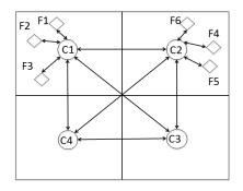
Fig. 2. An example RoboCup Rescue organization where the city is divided into four regions, with a manager (centers C1, C2, C3, and C4) responsible for each region. Agents assigned the role of extinguishing fires (fire brigades F1 to F6) are also shown for the C1 and C2 regions.
