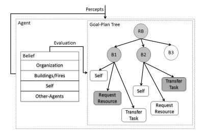
Fig. 4. Center OAA architecture (with an example goal-plan tree). Shown are a general Rescue Buildings (RB) goal and three goals specific to buildings on fire (B1, B2, and B3). Three plans are shown: extinguish building using the center's own resources, request resources from neighboring centers, and transfer the extinguish task to neighboring centers. Selected plans and goals are highlighted.
