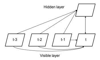
Figure 1: The architecture of a CRBM of order 3.
