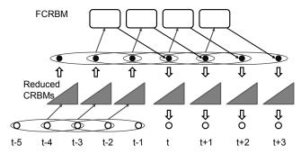
Figure 5: The generation process. A short motion sequence is input to the reduced CRBM, and the motion data is converted into the seed sequence of the FCRBM. Starting from this seed sequence, the FCRBM generates new data and uses it as new seed for further generations. The reduced CRBM takes the output of the FCRBM to construct motion data.
