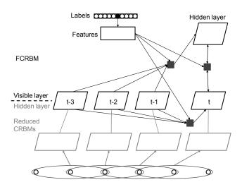
Figure 4: The architecture of the entire model. The reduced CRBM at the bottom layer is trained first, and the FCRBM then takes the approximate filtering distribution from the bottom layer as input to train its connections. There is a feature layer linked to the label nodes that propagates the label information to the model.
