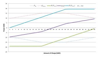
Figure 4: Graph showing the change in Preferred Operating Point (POP) and Advertised Regulation Capacities,  $P_{up}$  and  $P_{down}$  with the amount of charge in the EDV battery. Note that  $E_{cap} = 35kWh$ ,  $E_{min} = 5kWh$  and  $\delta t = 1hr$ .
