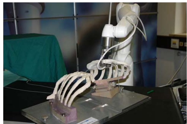
Fig. 1 3D Phantom Model including thorax framework, vascular system and surrounding tissue of the LITA and an universal robot with a monopolar blade electrode and an ultrasound probe mounted on it
