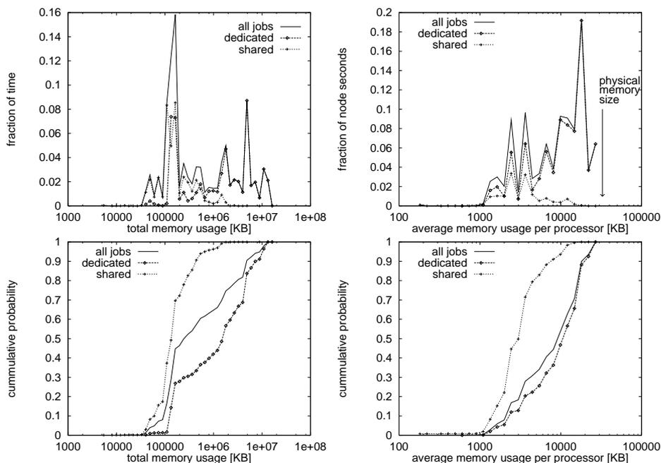
**Fig. 6.** Distributions of memory usage by jobs using dedicated or shared nodes. Left: total memory usage, weighted by job runtime. Right: average memory usage per processor, weighted by job runtime and number of processors. Top: pointwise distribution. Bottom: cumulative distribution (each normalized independently).
