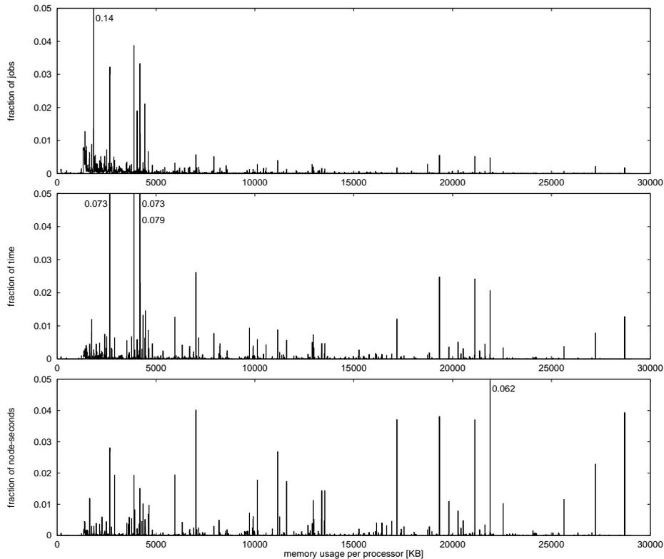
**Fig. 2.** *The distribution of per-processor memory usage, using a linear scale and buckets of 10 KB. In the top plot, all jobs have equal weight. In the middle, jobs are weighted according to their run time. The bottom plot shows the distribution for individual processors, which is equivalent to weighing the jobs according to the product of runtime and degree of parallelism.*
