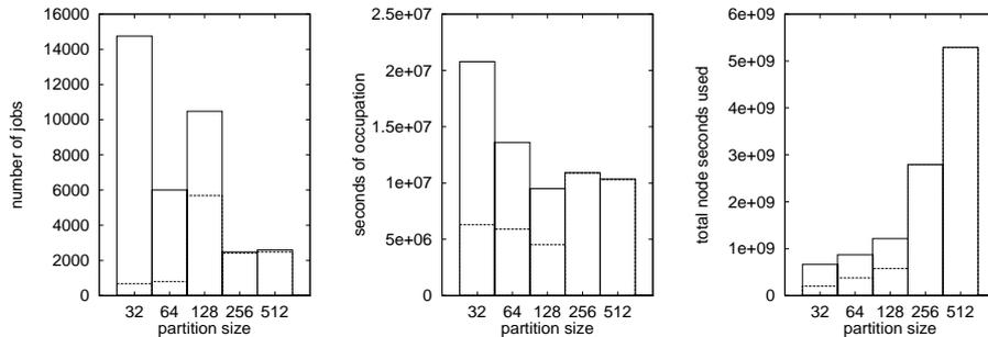
Fig. 1. Histograms of job sizes in the analyzed log. In the left graph, all jobs have equal weights. In the middle, jobs are weighted by their runtime. At right, jobs are weighted by the product of runtime and parallelism, which is equivalent to counting node-seconds.
