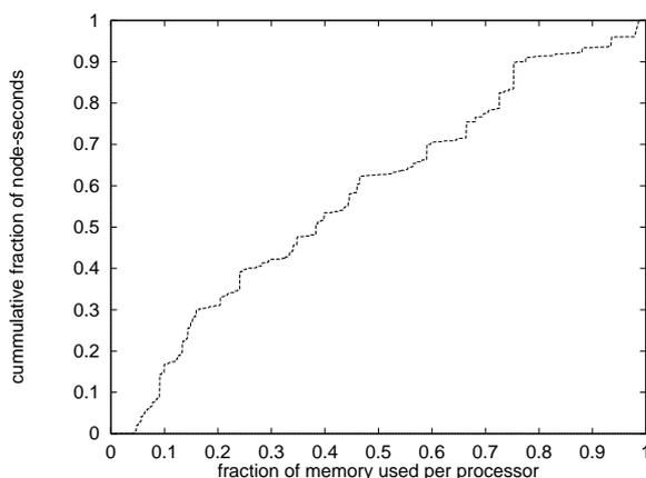
**Fig. 9.** Cumulative distribution of per-processor memory usage, weighted by runtime and number of processors.
