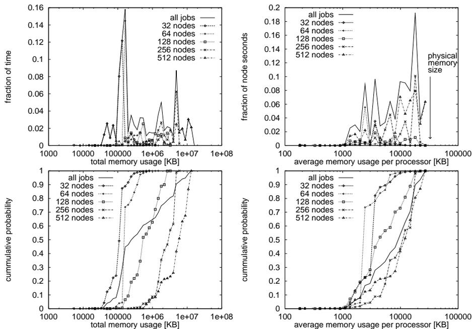
**Fig. 5.** Distributions of memory usage by all jobs and jobs of different sizes. Left: total memory usage, weighted by job runtime. Right: average memory usage per processor, weighted by job runtime and number of processors. Top: pointwise distribution. Bottom: cumulative distribution (each normalized independently).
