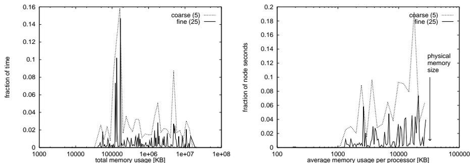
**Fig. 3.** Distributions of memory usage using coarse and fine bucket sizes.
