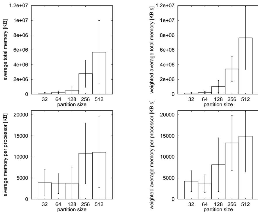
**Fig. 4.** Average memory usage by jobs of different sizes. The top graphs are for total memory usage, and the bottom ones for per-processor usage. In each pair, the left graph is a simple average, while the right one is weighted by time. The error bars denote the standard deviation.
