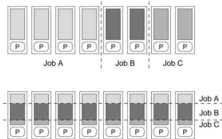
**Fig. 10.** With space slicing, processor allocation dictates memory allocation due to the “vertical” partitioning (top). With gang scheduling, memory is partitioned “horizontally”, so memory allocation is decoupled from processor allocation (bottom).
