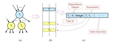
Fig. 1. (a) A portion of a task dependency graph. (b) The corresponding representation of the global task list (GL). (c) The data of element  $T_i$  in the GL.
