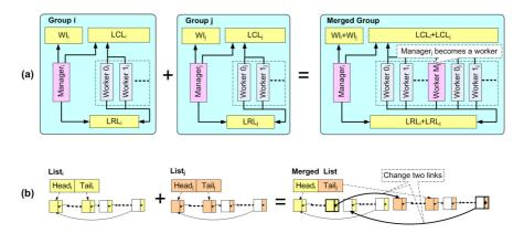
Fig. 3. (a) Merge  $Group_i$  and  $Group_j$ . (b) Merge circular lists  $List_i$  and  $List_j$ . The head (tail) points to the first (last) tasks stored in the list. The blank elements have no task stored yet.
