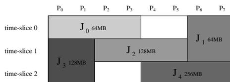
**Fig. 3.** Empty slot utilization with GS
