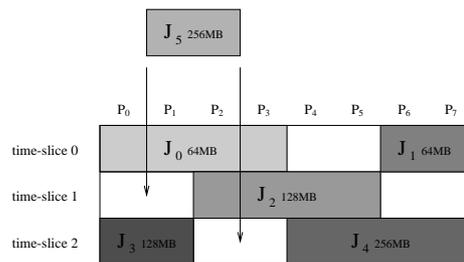
**Fig. 2.** Ousterhout Matrix of an 8-Processor System with 512-MB Memory/Processor and Multiprogramming Level of 3.
