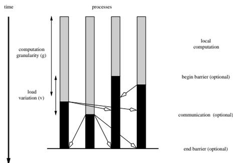
Fig. 4. Overlap of Computation and Communication
