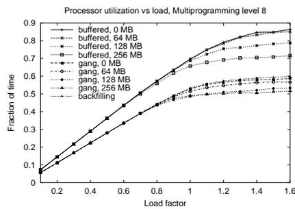
Fig. 9. Processor Utilization versus Load for BCS and BGS.
