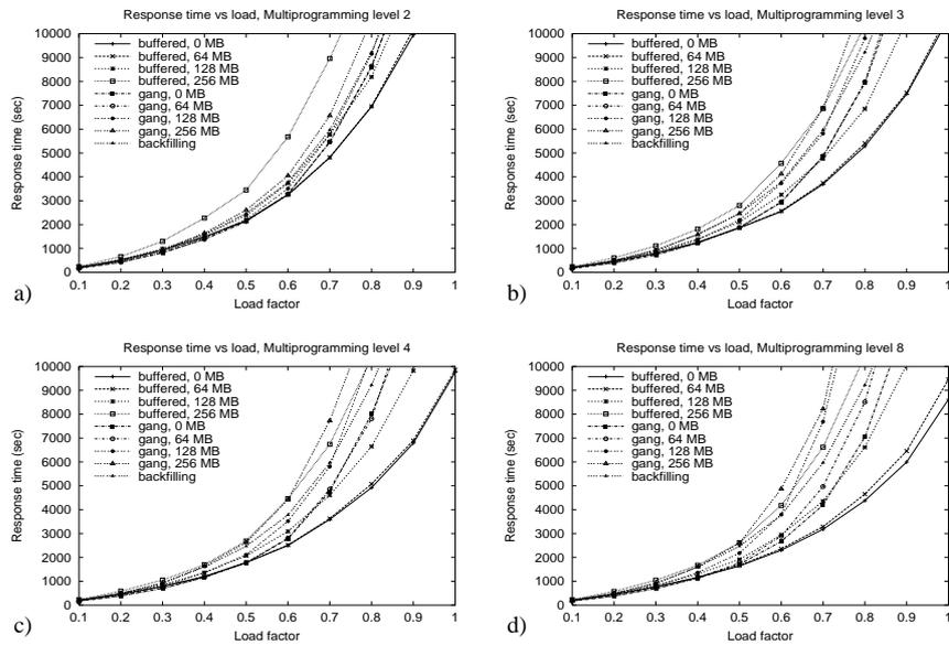
Fig. 6. Response time versus load for various MPLs. The graphs compare BCS with BF and BGS.
