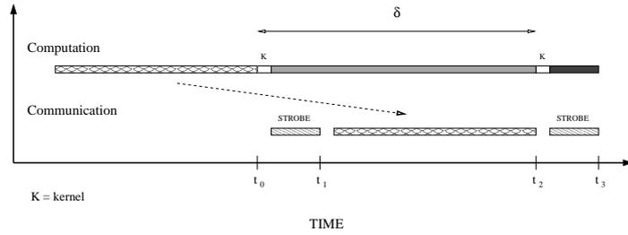
**Fig. 1.** Scheduling Computation and Communication. Communication accumulated in the time-slice up to  $t_0$  is downloaded into the network between  $t_1$  and  $t_2$  (after the heart beat).  $\delta \equiv$  length of a time-slice =  $t_2 - t_0$ .
