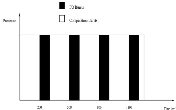
**Fig. 1.** I/O bound job with one I/O working set
