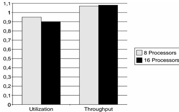
**Fig. 8.** Evaluation of the spin control mechanism - IO/Msg Workload
