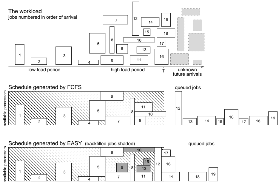
Fig. 1. Illustration of a sequence of parallel jobs (the workload) and how it would be scheduled by FCFS and EASY up to time T.
