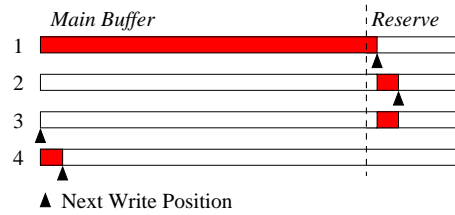
Figure 1: The four steps of the flush operation: (1) The log buffer reaches the low-water mark and wakes up the dump thread. (2) Thread writes the data between the beginning of the buffer and the current position, possibly causing new events to be logged to the reserve part. (3) Atomically resetting the buffer’s current position (with interrupts disabled). (4) Events from the reserve part are flushed to disk, possibly causing new events to be logged at the beginning of the buffer.
