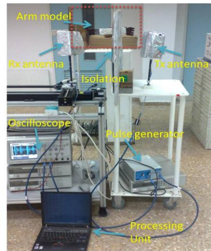
Figure 3. UWB sensor node prototype and arm model in the back. The arm model in the back was moving back and forth from and to the UWB acquisition system in a way that maximized the reflection surface.
