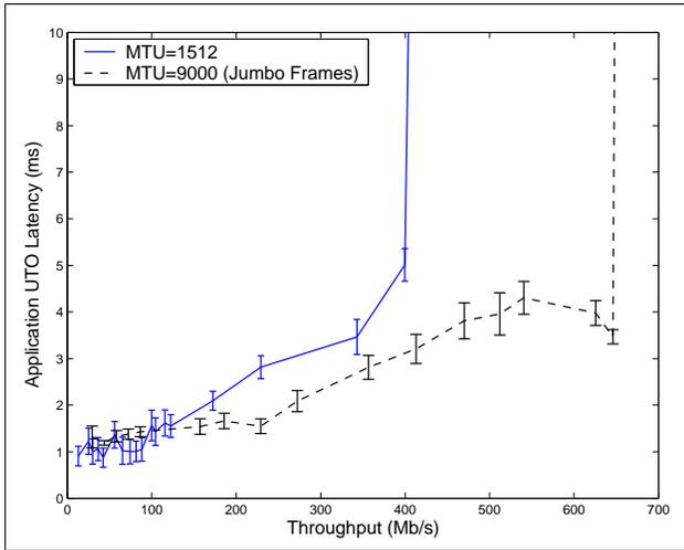
Fig. 7. Latency vs. Throughput for different MTU sizes
