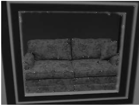
Figure 4: The output of the Harris corner detector [8] on one image. The features used in our experiments are the corners of the internal frame in the aperture.
