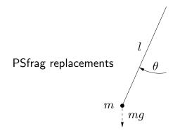
2nd order nonlinear DE  $ml^2\ddot{\theta} = -lmg\sin\theta$ rewrite as first order DE with state  $x = \begin{bmatrix} \theta \\ \dot{\theta} \end{bmatrix}$ :
