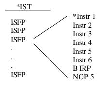
When the CPU begins processing an interrupt, the interrupt service table (IST) is used. The IST is a table of fetch packets that contain code for servicing the interrupts. The IST consists of 16 consecutive fetch packets. Each interrupt service fetch packet (ISFP) contains eight instructions used to service the interrupt. One of the instructions is a branch to the interrupt return pointer instruction (B IRP).
