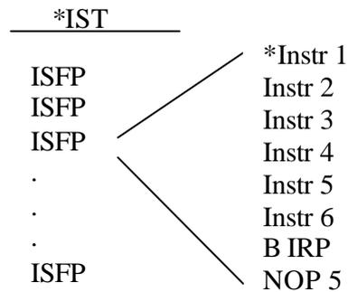
When the CPU begins processing an interrupt, the interrupt service table (IST) is used. The IST is a table of fetch packets that contain code for servicing the interrupts. The IST consists of 16 consecutive fetch packets. Each interrupt service fetch packet (ISFP) contains eight instructions used to service the interrupt. One of the instructions is a branch to the interrupt return pointer instruction (B IRP).
