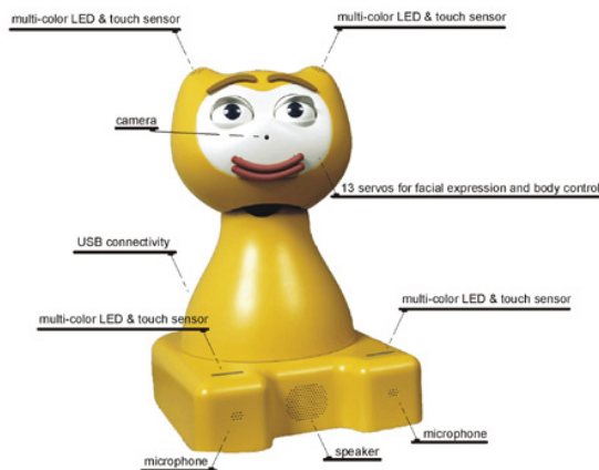
Figure 1. Hardware setup of the “iCat”.
