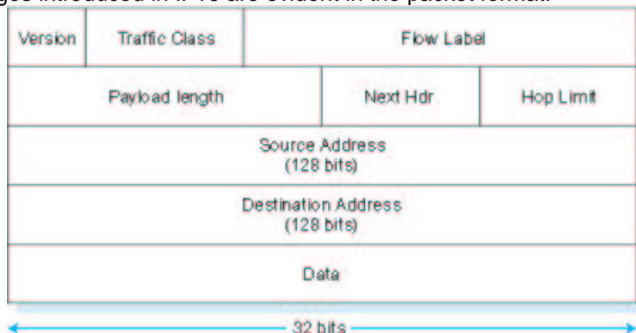
Figure 4.40: IPv6 packet format
