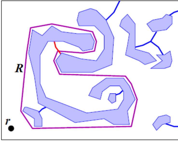
Figure 13: A shortest path map SPM(r) for F with k = 8 obstacles (blue), showing the bisector set B (red), which has one SPM-vertex, 7 connected components, and 9 arcs. R is the shortest cycle corresponding to the red bisector arc. Other bisector arcs are blue, having become part of the obstacle set for F' .
